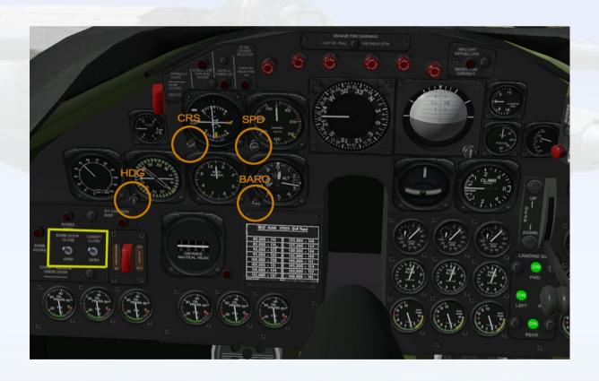
On the right side of the cockpit, the pilot's console carries all the switches needed for lights, autopilot, electrics and fuel cutoff switches, shown in the yellow rectangle below.
