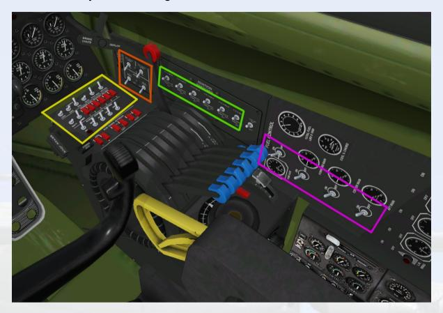
The orange rectangle highlights the four generator switches. The row of switches in the green rectangle are the starter switches. The purple rectangle highlights the fuel pump switches, these are not needed for the operation of the aircraft and are only included for authenticity.
