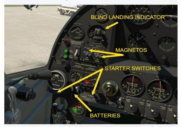
The 'Blind Landing Indicator', also know as the Lorentz Instrument is set up in this simulation as a LOC/DME indicator.
