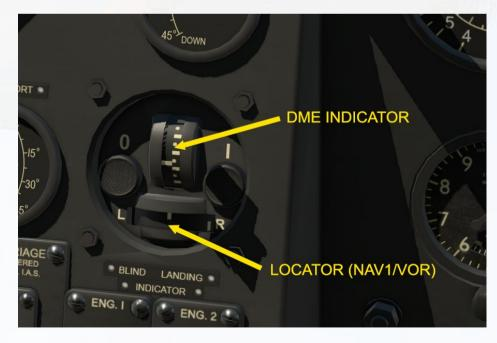
The upper instrument measures distance in nautical miles to the presently tuned NAV1 or TACAN station. The increments are 5 nm each, the needle will move downwards the closer the aircraft is to the station.
