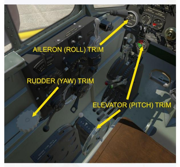
The rudder and aileron trim knobs are easy to manipulate with the mouse cursor, the elevator trim wheel however is awkward to use given its orientation and position relative to the user. It is advised that the joystick buttons are used for elevator trim.
