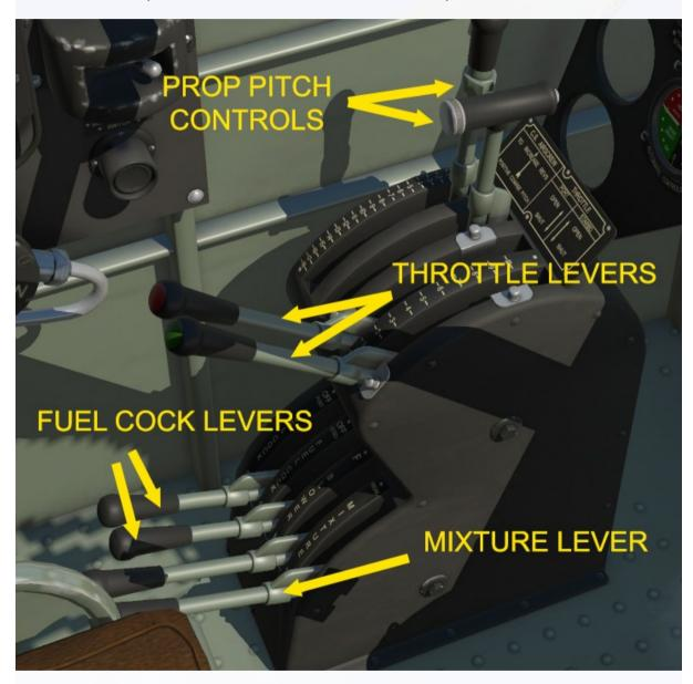
The mixture lever controls both engines, the down position (RICH) is the normal setting for running engines. It can be raised to about half way to waeken the mixture, any higher and the engines will stall. The two fuel cock levers control the fuel supply to left and right engines. The
