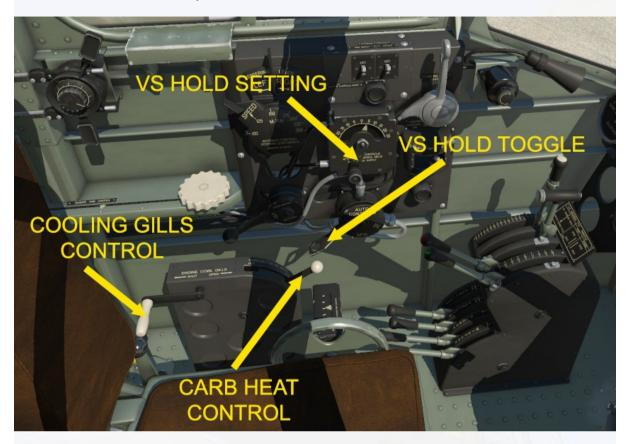
The cooling gills (cowl flaps) lever is operated by click-and-hold, the lever will rotate and both engines' gills will open/close as long as the lever is turning. The carb heat lever is self-explanatory. It will be necessary to raise the arm rest out of the way to access these levers, do this by clicking on any part of it.
