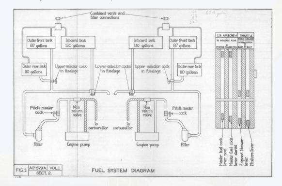
In the real aircraft, the fuel gauges can read the contents of either left or right tanks by turning the associated left/right selector knob. It was not possible to replicate this function in X-Plane so the gauges read only the left side. However, as the tanks drain uniformly, there would be no difference under normal circumstances between the contents of either side. Capacities are in US gallons (XP limitation) rather than Imperial gallons.
