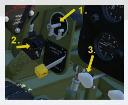
1) Magneto Switches (standard L, R, start) and Master Ignition Switch.
