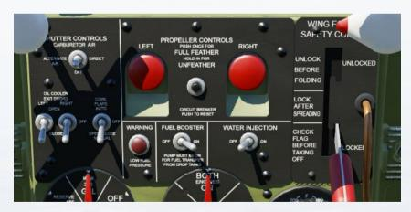
1) Shutter Controls Switch. This functions as the carb heater and should always be ON unless the environment air temperature is high.
