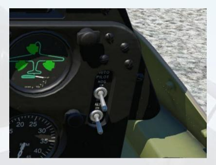
The small oval area on the right side of the panel is normally blank on the F7F-3 day fighter, its purpose being to accommodate three lamps associated with the radar altimeter system of the night fighter version. In this model, this area to house a pair of toggle switches used to activate Altitude Hold (ALT) and Heading Hold (HDG) for the convenience of the user.
