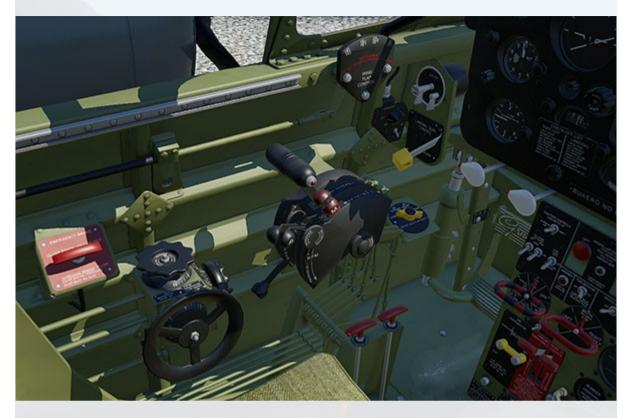
The main features on the left side are flaps & gear operation, the throttle quadrant, trim controls, magneto switches and emergency brake handle. Additional points of interest are outlined below:
