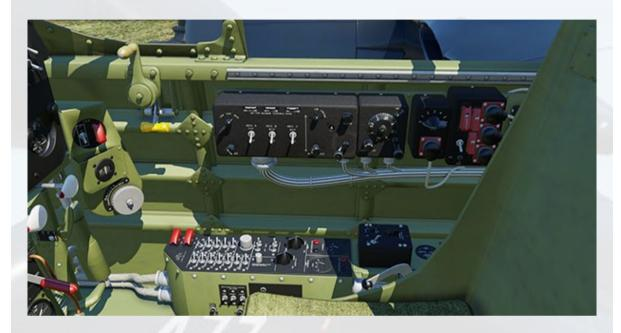
The main features on the right side are canopy handle, electrical systems control, tail hook handle and rudder booster handle. Additional points of interest are outlined below:
