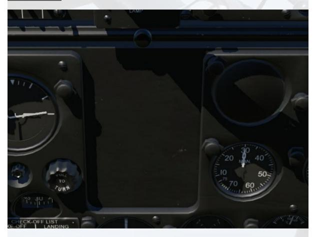
There is not a 'missing gauge' in the panel, The empty gauge hole and adjacent rectangular area are authentic. The rectangular area is where the pilot's radar scope is fitted on the 2-seater night fighter Tigercat (F7F-3N). The gauge would be a radar altimeter on the night fighter, Grumman elected to not use the space for another instrument. The 'Push To Turn' knob on the left is also part of the radar altimeter system and is used in this simulation to toggle the control stick visibility.
