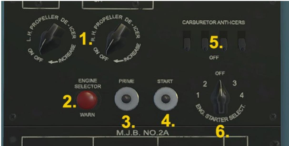
1. Propeller De-Icing Switches
